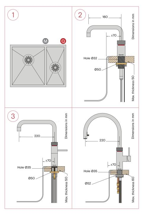
**1. Select position Nordic single tap** Select a suitable position for the Nordic single tap based on the type of sink and position of the mixer tap.
